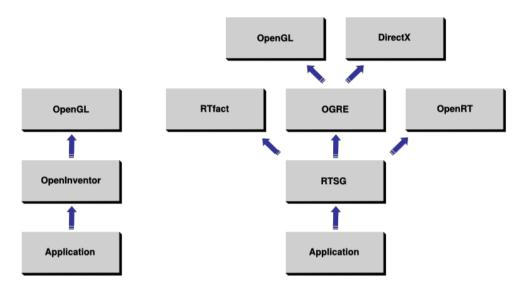
Figure 2: Comparison of OpenInventor (left) and RTSG (right) application scheme
