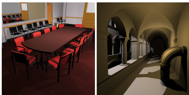
Figure 3: Scenes rendered at a 1024^2 resolution on a mobile Core 2 Duo processor. Left: CONFERENCE with a mirror and two light sources (8.2 fps). Right: SPONZA with three light sources (7.3 fps).
