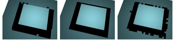
**Figure 4:** The effect of a scan line processing order (left image) on the approximation error for non-adaptive quantization. The shadows from the cube appear shifted towards the bottom right. The right image uses random order, and the middle one is ground-truth.
