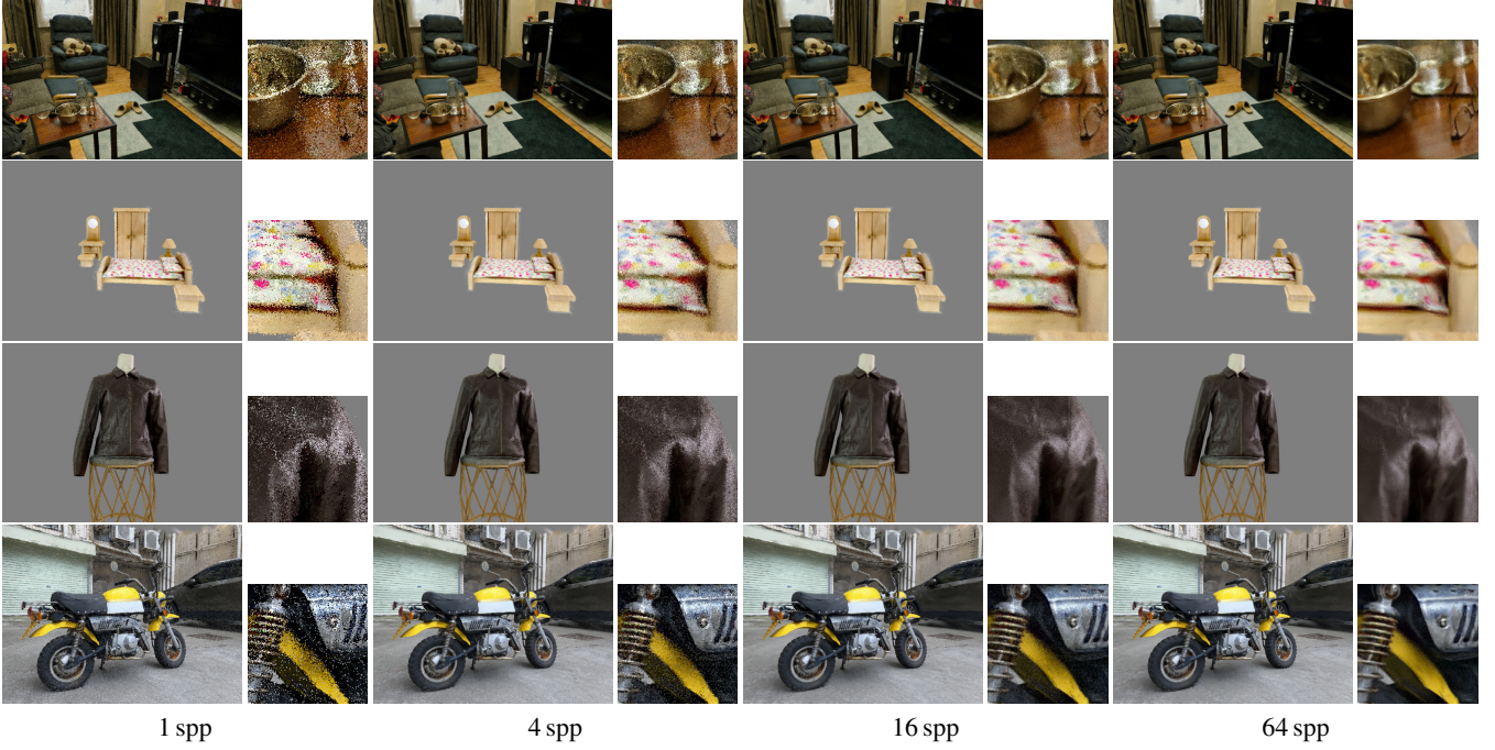
Figure 6: Convergence of our method. Although our stochastic binary opacity introduces Monte Carlo noise, it converges very fast. For all assets we tested, 1 spp already produces plausible rendering, and most noise is eliminated with 64 spp or less.
